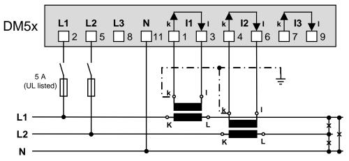
Three wire system, balanced load, phase-shift current measurement L1, voltage measurement L1-L2
