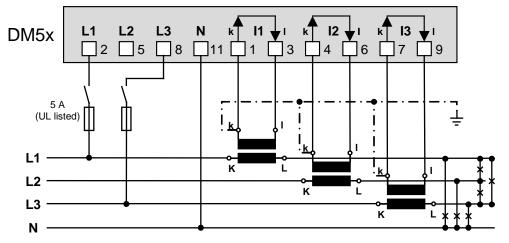
• With current and 2 single-pole isolated voltage transformers
